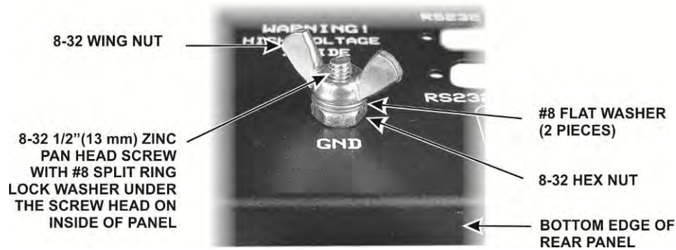
Figure 21. Installing the Rear Panel Ground Lug.
