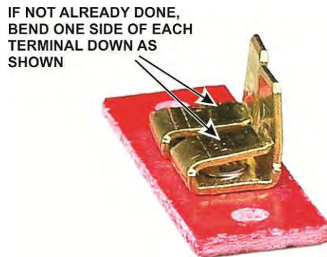
Figure 17. Preparing the Terminal Strip Board.
