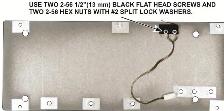
Figure 12. Mounting the Interlock Switch on the Left Side Panel.
