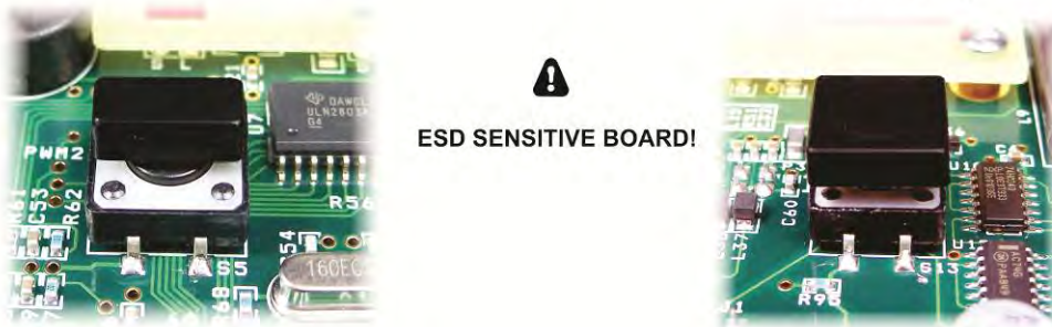
Figure 57. Installing Key Caps on Front Panel Board.
